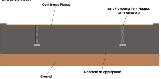
Overall Thickness of Plaque - ~12mm Thickness of Plaque where text and detail is recessed - ~10mm Protrusion Depth of Bolts - ~50mm
